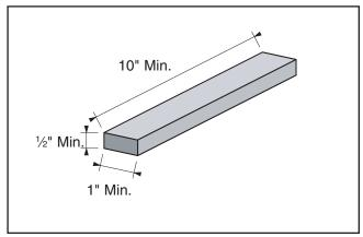
**Figure 21.** Minimum dimensions for surface planing.
